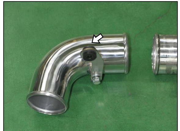
Reuse the factory grommets
