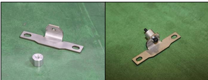
P4: Intercooler bracket No.1 P17: Collar P26: M6 Hex Socket Head Cap Bolt L=35 P27: M6 Spring Lock Washer P28: M6 Flat Washer
