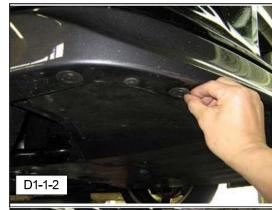
(2) Remove the inner fenders (Left and right side). (Dia.1-1-3)
