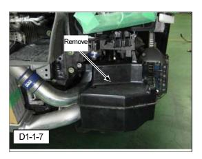
(8) Remove the undercover, mid pipe, and heat shield. If the factory exhaust system is used, remove the main muffler section as well. (Dia.1-1-8)
