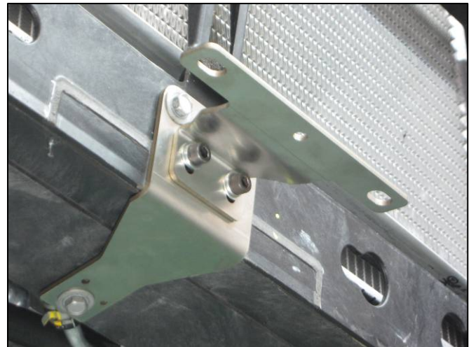
Secure the flange nut using the factory bolts.
