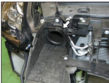
Remove the air funnel from both sides.
